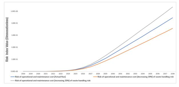
Figure 9: Sensitivity Test Analysis Patterns of Operational and Maintenance Cost Risk if Waste Handling Risk Change
