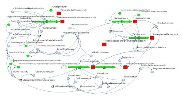
Figure 3: Stock and Flow Diagram of Environmental, Health and Safety Risks
