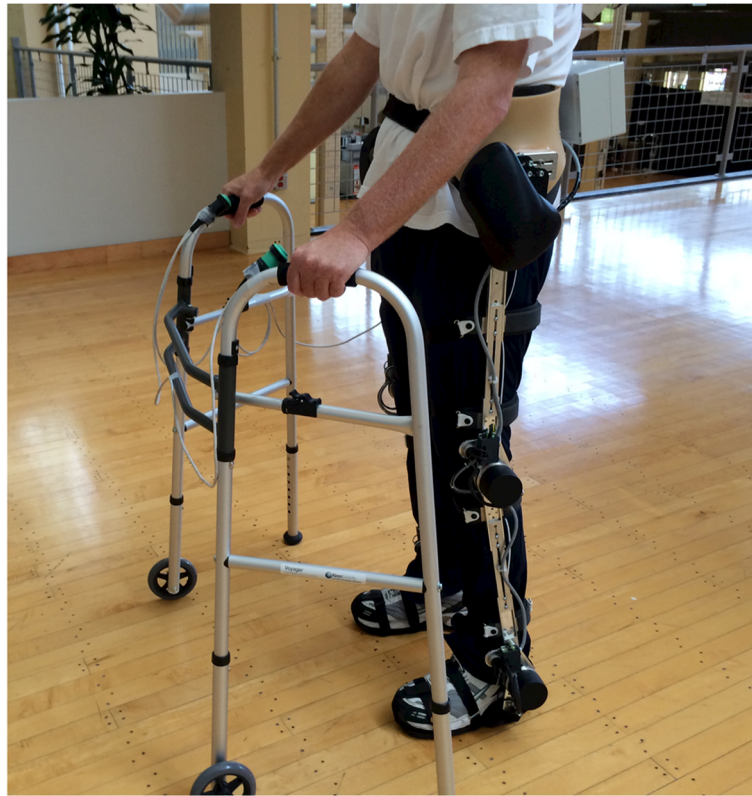
Fig. 4 Stroke patient using H2 exoskeleton at the beginning of one training session
