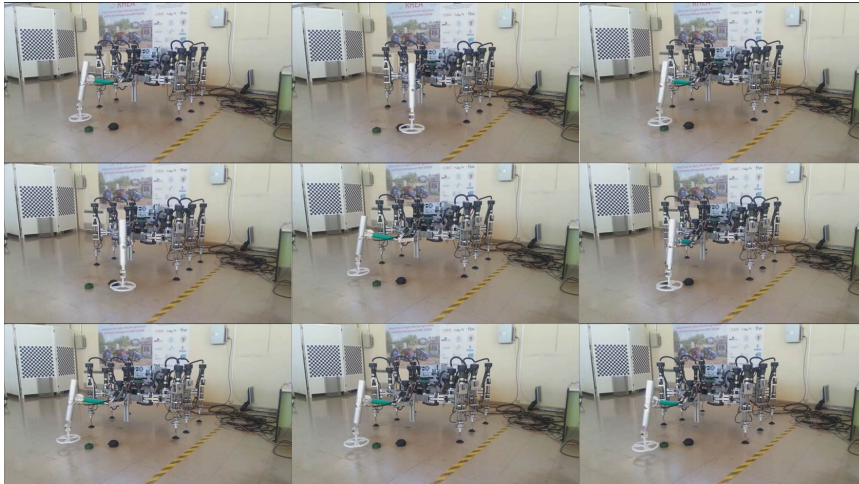
Figure 6. Photographic sequence (left to right and up to down) of a gait pattern of the hexapod robot.
