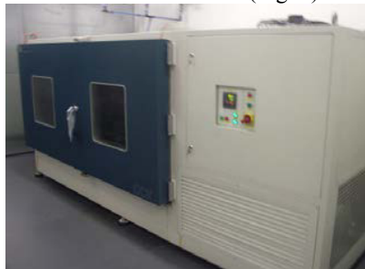
Fig. 4. Pictures of relative humidity climatic chambers in CENER
