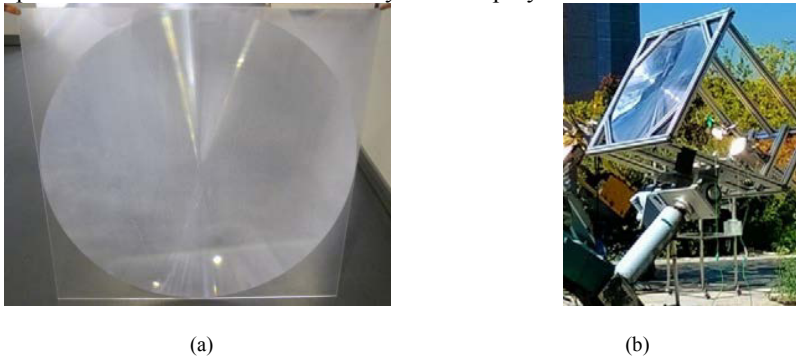
Fig. 3. Pictures of the Fresnel lenses used for thermal shock test (a) un-mounted in CENER (b) on solar tracker in CSIC-CENIM
