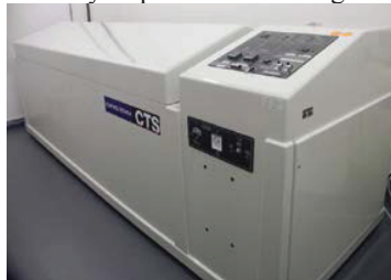
Fig. 2. Picture of the chamber used for salt mist test at CENER.
