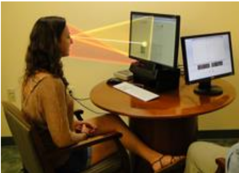
Figure 5.4 Infrared light emitted from eye tracker
