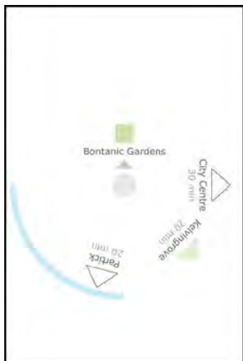
Fig. 5.18 The fourth FS design, FS#4. Here, the user's location is denoted by the middle circle. A nearby park is denoted by the green square. Around the edge, we see a river represented by a blue line and the direction of districts denoted by triangles.
