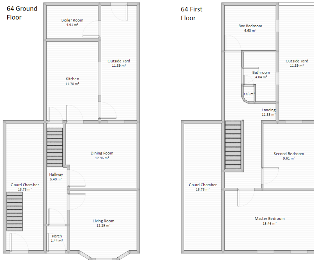
Figure 3-2 Test house 64 and guard chamber floor plan (house 63 is identical with the exception of the guard chamber located to the right side of the building). Ground floor plan is on the left of the figure and 1 st floor plan is on the right of the figure.
