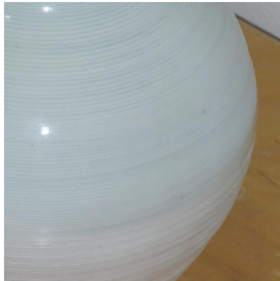
Fig. 2.9 close up of extrusion striations from fig 2.8
