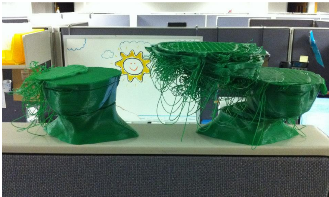
Fig. 1.4. Print errors using Freeform Fabrication (FFF)
