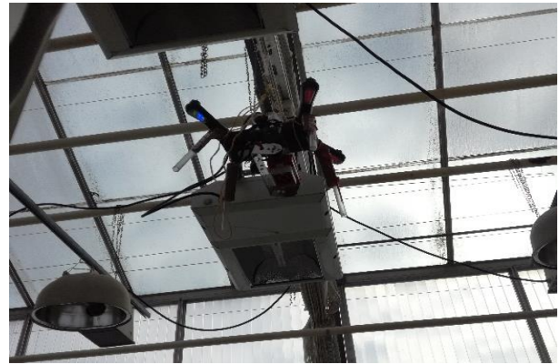
Figure 3. Multispectral camera being used to capture data in the greenhouse. The camera was connected to a drone for power and hang to the roof of the greenhouse by cables to capture the pot of cassava on the bench.
