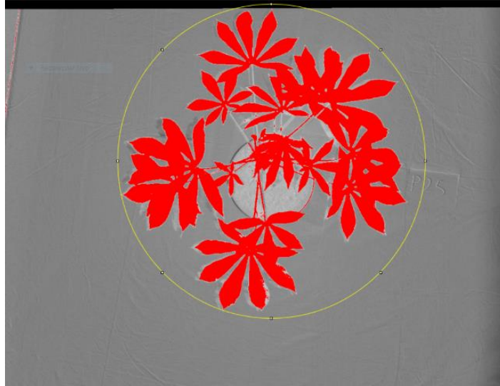
Figure 9. Selection of plant area using a threshold after NDVI calculation. The red portion shows the area which was detected by the ImageJ as leaves using the threshold. The average digital number of the selected region was recorded as the NDVI of the plant.
