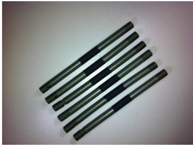
Fig 1. Anode supported mT-SOFCs using LSM-YSZ for the cathode
