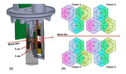
**Figure 1.** Sketch of the experimental setup. The position of the DSSSD's with respect to the target (a) and the position of the MINIBALL clusters with respect to the beam (b).
