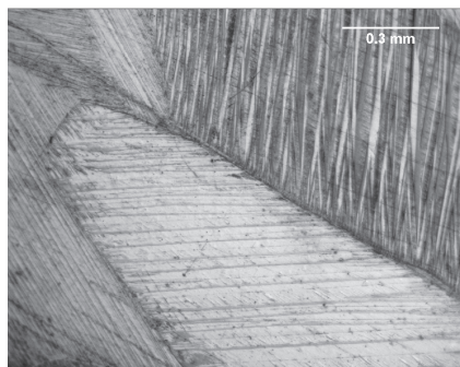
Fig. 1 The grain structure and martensitic morphology of Ni-Fe(Co)-Ga alloy. The black spots inside of the grains and their colonies on the grain boundaries represent precipitates of gamma-phase (see text for details).
