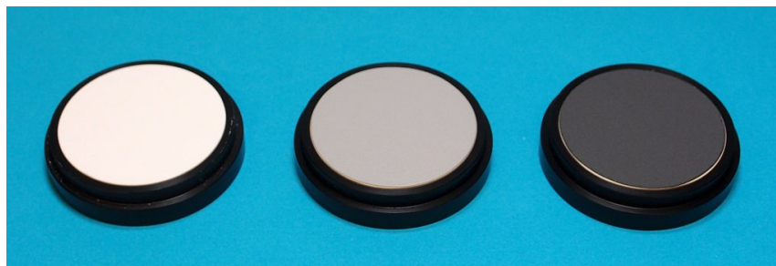
Figure 8. Diffuse matt ceramic grey scale standards, containing three different reflectances of 88 % white, 40 % grey and 5 % deep grey
