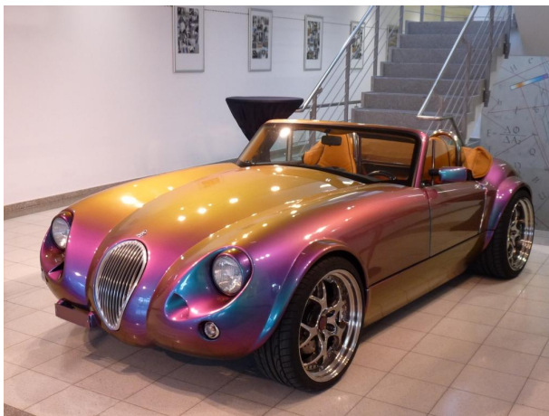
Figure 2. Car painted with a goniochromatic varnishing, according to the visual perspective and the light conditions, the color impression changes
