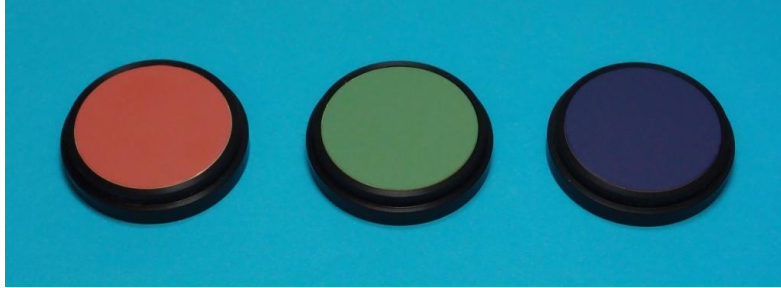
Figure 9. Diffuse matt ceramic color standards, containing three different colors, red, green and blue
