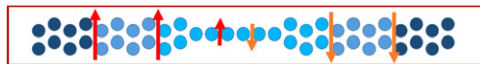
Figure 17. Sketch of the EM setups used in the calculation of spin-resolved transport through nickel electrodes that corresponds to the EM unit cell shown in figure 5. The scattering region is shown in light blue, the first PL is shown in grayish blue, and the second PL is shown in dark blue. The second PL is followed by vacuum.
