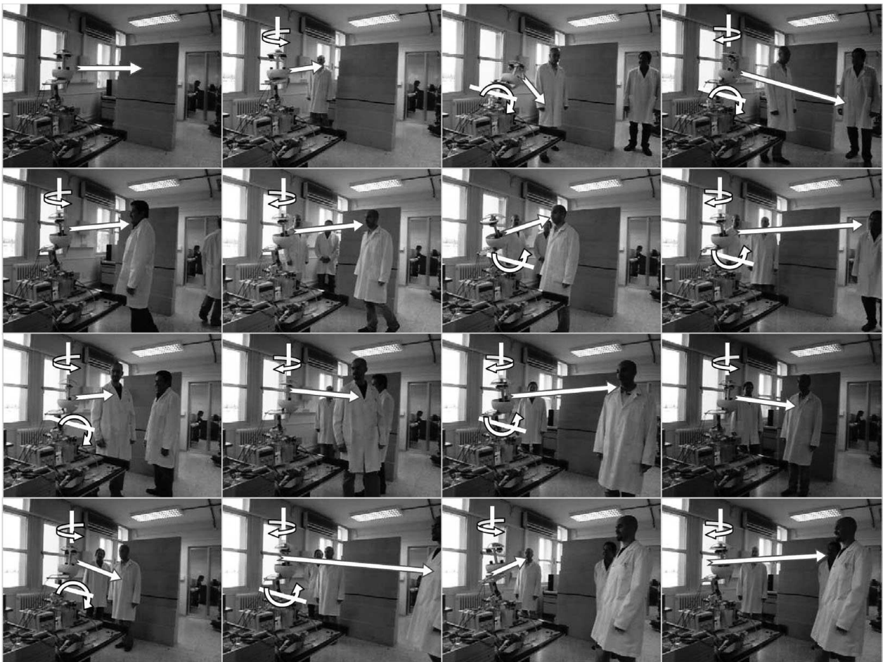
Fig. 15. Experimental testing of the implemented visual servoing algorithm to detect moving objects using omnidirectional stereovision system.
