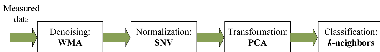
Figure 12. Optimal algorithms for the four-step signal-processing chain designed to deal with low-accurate narrowband fluorescence measurements.
