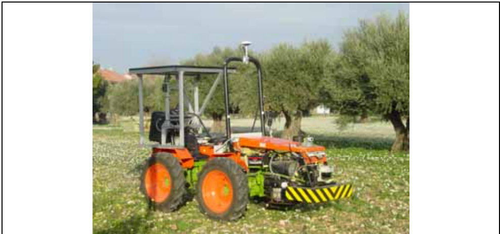
Fig. 1. Experimental vehicle: robot tractor DEDALO
