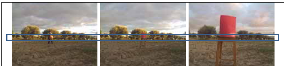
Fig. 7. Red card detected by the laser at 8, 4 and 1 m. distance from the vehicle, within the limited visual area inscribed in the blue frame.
