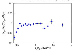
FIG. 5 (color online). Asymmetry between the numbers of reconstructed  $D^{*+}$  and  $D^{*-}$  candidates as a function of the soft pion's  $p_T$ .
