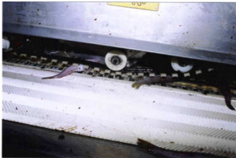
Fig. 7. BAADER 424 Cont. The uneven cuts of P. Ramsayi bodies at the BAADER 424 is caused by the small size of the fish, the small fishes do not hold to the conveyor belt, when the belt begins to move further the fish position changes causing irregular cuts.
