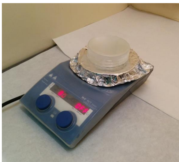
Figure 9. Picture of the Petri dish set up for reduction of thin films in hydrazine monohydrate.
