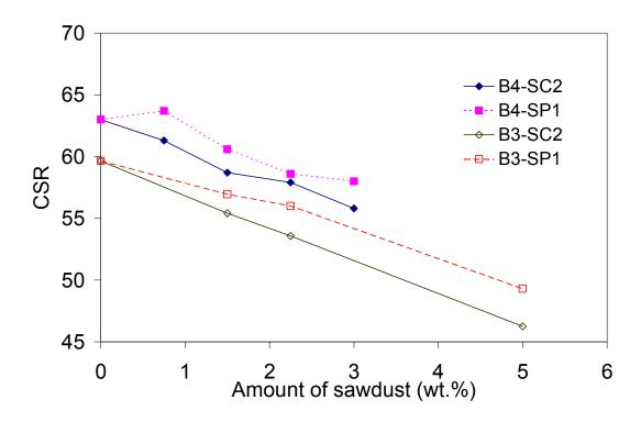
Figure 7. Variation of the CRI and CSR indices of the cokes containing various amounts of sawdust.
