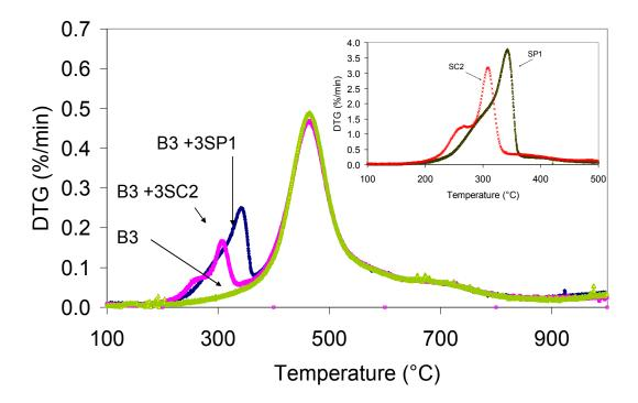
Figure 3. Thermogravimetric curves corresponding to the industrial coal blend B3 and the mixtures with sawdusts SP1 and SC2.
