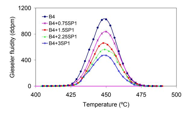
Figure 1. Gieseler curves of the industrial blend B4 with various amounts of sawdusts SP1 and SC2.
