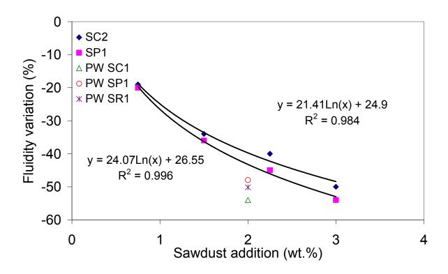
Figure 2. Variation of the Gieseler fluidity of the mixtures of blend B4 with sawdust with respect to that of B4. PW SC1, PW SP1 and PW SR1 correspond to data from ref. 5.
