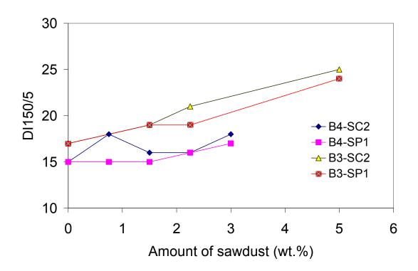
Figure 6. Variation of the JIS indices with the amount of sawdust added to the industrial coal blends B3 and B4.
