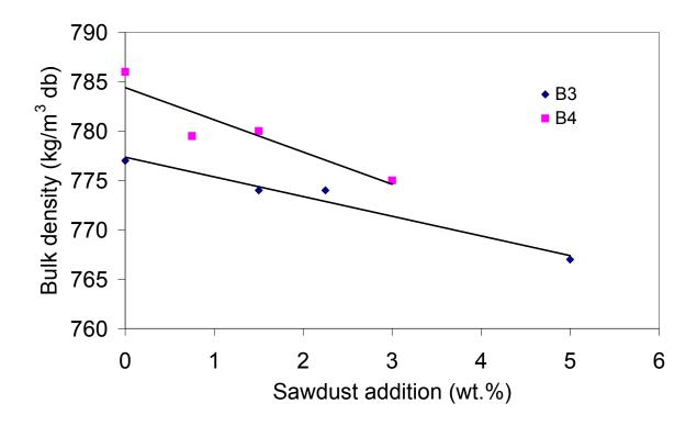
Figure 5. Variation of bulk density of the charge in the coking oven with SC2 addition.
