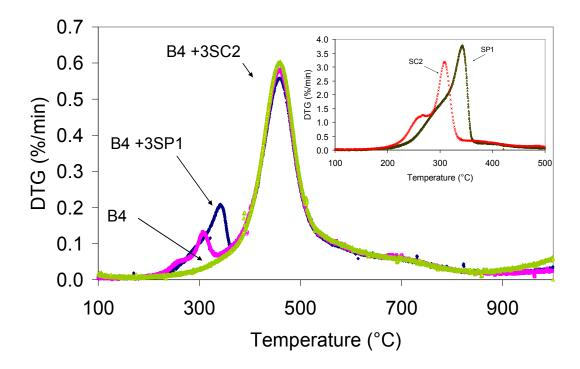
Figure 4. Thermogravimetric curves corresponding to the industrial coal blend B4 and the mixtures with sawdusts SP1 and SC2.
