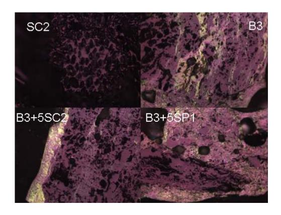
Figure 8. Microphotographs of the char obtained at 900 °C from SC2 and of the cokes from the industrial coal blend B3 and their blends with 5wt% of SC2 and SP1. Magnification: x50.
