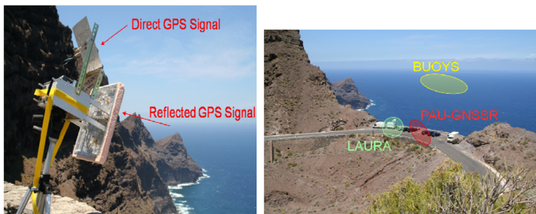
Fig. 17 The PAU (Passive Advanced Unit) GNSS-R receiver and the instruments deployed, pointing at the test zone in which the buoys were moored to obtain ground-truth data.
