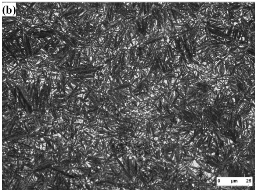
Figure 7. Optical microscopy micrographs showing examples of the 1C alloy bainitic microstructure obtained by isothermal transformation (a) 220°C and (b) 300°C.
