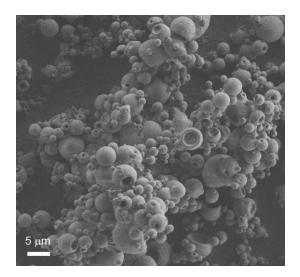
Figure 1. Hollow MOF superstructures obtained by spray-drying.
