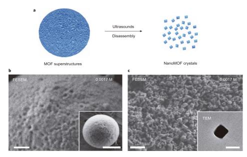
Figure 2. a, Schematic showing the disassembly of the HKUST-1 superstructures upon sonication to form well-dispersed, discrete nanoHKUST-1 crystals. b, Representative FESEM and TEM (insets) images of the HKUST-1 superstructures (b) and corresponding disassembled nanoHKUST-1 crystals (c).
