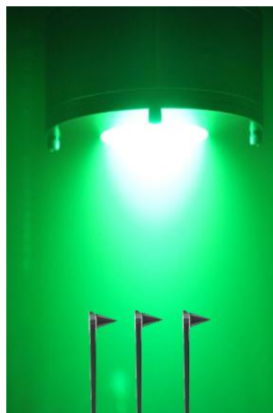
Figure 4.2: Deposition of the magnetic coating. Commercial AFM tips are sputter-coated with a polycrystalline Co film.
