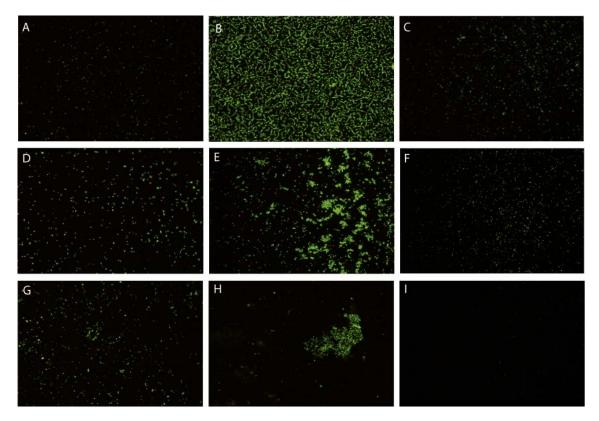
Figure 3. Epifluorescence images of all strains studied on AISI 304 SS, showing the distribution of
