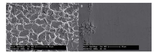
439 Figure 2. SEM micrographs of (A) AISI 304 SS and (B) AISI 316 SS surfaces. Micrographs show
