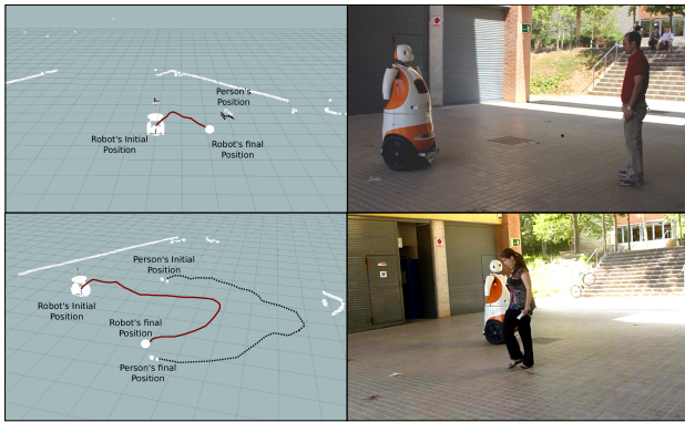
Fig. 6. Tibi Starts an Interaction. The robot approaches two people and begins an interaction with them. Top: The person is waiting for Tibi. Bottom: The person is moving and Tibi follows her and invites her.
