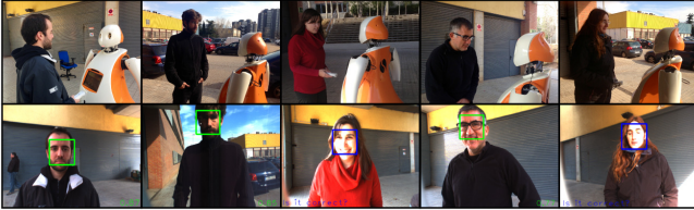
Fig. 8. Face Recognition. Top: People interacting with the Tibi robot. Bottom: Tibi's field of vision. Face detections are represented by green boxes, whereas blue ones indicate that the system requires the human assistance.
