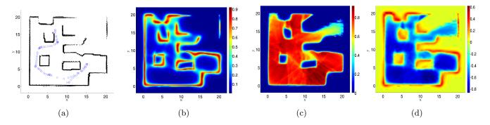
Figure 1: A regressed information distribution map for the Cave environment, size of  $20m \times 20m$ . a) Map of explored area, where the blue circles are robot poses and the black points are relevant laser scans. b) The obstacle distribution map  $\Lambda_o$ . c) The free space distribution map  $\Lambda_f$ . d) The overall information distribution map  $\Lambda$ . For  $\Lambda_o$ ,  $\Lambda_f$ , data is locally normalized between 0 and 1 at each iteration.
