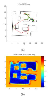
Figure 4: a) Exploration in Cave map, size of  $20m \times 20m$ . In this experiment, loop closures detected during Pose SLAM caused small rotations in the map. b) Final information distribution map; in information form, these sharp loop-closure changes are better absorbed in its final representation. In spite of the sparse measurements at some locations, at the end of the experiment the whole map is completely explored based on the information map.
