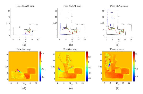
Figure 2: Evolution of the frontier surface in the Cave map during an exploration experiment. a-c) In pose SLAM maps red lines and points show the planned path and the robot poses, respectively. Green lines indicate detected loop-closure. d-f) The frontier map facilitates exploration goal extractions. Negative values show information variations between known and unknown areas, whereas positive values represent information variations around obstacles. Maps are non-dimensional.
