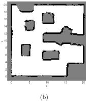
Figure 3: The Final occupancy grid maps; a) exploration with the grid-based method and b) exploration in information distribution map. Inferring the information distribution map with GP regression leads to a partially incomplete equivalent occupancy grid map. See Fig. 4 for a completed experiment with GP regression.
