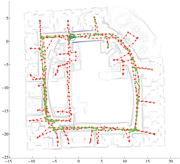
Figure 7: Filtered trajectory using encoder and laser odometry of the Intel data set. The blue arrow indicates the final pose of the robot and the black ellipse the associated covariance at a 95% confidence level.
