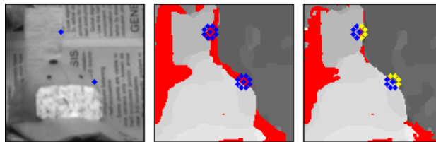
Fig. 3. Application of masks to scenes with occlusions. Left to right: reference image, a depth map after one iteration, and a posterior refinement using masks. Enabled grid points are shown in blue, and disabled grid points are drawn in black. We show a simplified grid of 9 points, for simplicity.
