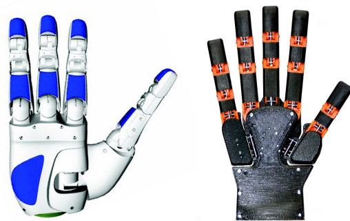
Fig. 1. Different robotic hand designs, the Schunk Anthropomorphic hand, based on the DLR II hand, with four fingers (left), and THE first hand developed at the Centro E. Piaggio with five fingers (right).
