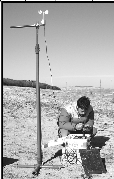
Figure 1: Measurement equipment: Cup anemometer on a tripod connected to a data logger fed by a solar panel.
