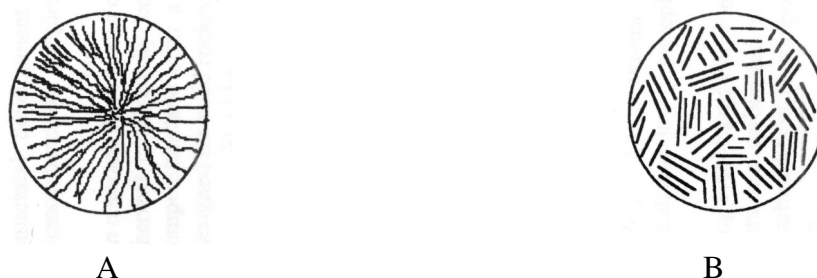
Fig. 22. Scheme of the fibre cross section of (a) an anisotropic (PAN type) CF and (b) an isotropic (pitch type) CF
