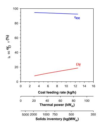
Fig. 11. Effect of the coal feeding rate on the predicted values for  $CO_2$  capture ( $\eta_{CC}$ ) and oxygen demand ( $\Omega_T$ ).Reference test VII-5.
