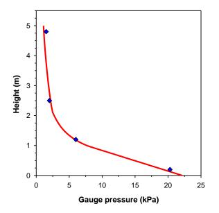
**Fig. 5.** Pressure profile from the experiment VII-5. Continuous lines: model predictions; Symbols: experimental results.
