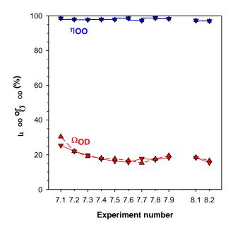
Fig. 7. Oxygen demand in the fuel reactor ( $\Omega_{OD}$ ) and oxide oxygen capture efficiency ( $\eta_{OO}$ ) obtained for tests VII and VIII evaluated in this work. Continuous lines: experimental results; Dashed lines: model predictions.
