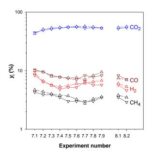
Fig. 6. Dry concentration of  $CO_2$ , CO,  $H_2$  and  $CH_4$  at the fuel reactor exit obtained for tests VII and VIII evaluated in this work. Continuous lines: experimental results; Dashed lines: model predictions.
