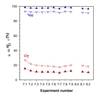
Fig. 9. CO<sub>2</sub> capture effiency ( $\eta_{CC}$ ) and total oxygen demand ( $\Omega_T$ ) predicted by the model for the different experimental conditions in VII and VIII tests. Solid symbols: for experimental  $\eta_{SF}$ ; Empty symbols: for  $\eta_{SF} = 100\%$ .
