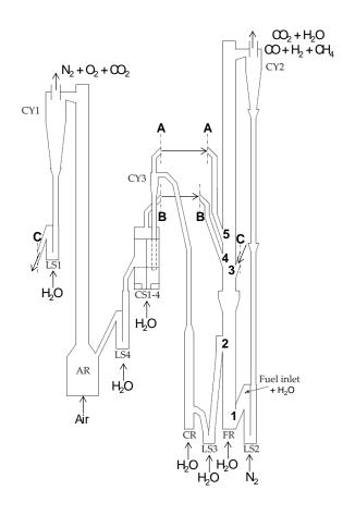
Fig. 3. Schematic picture of the 100 kW<sub>th</sub> CLC system at Chalmers UT (Markström et al., 2013b). Numbers 1-5 indicate modifications in the model compared to the model concept for the 1 MW<sub>th</sub> unit at TU Darmstadt (Abad et al., 2013.
