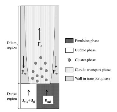
**Fig. 2.** Gas and solids distribution in the fuel reactor, considered as a high-velocity fluidized bed reactor.
