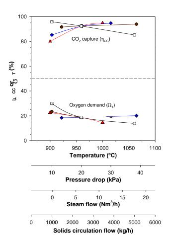
**Fig. 10.** Effect of operating conditions (temperature:  $\clubsuit$ ; pressure drop:  $\clubsuit$ ; steam flow:  $\clubsuit$ ; solids circulation flow:  $\blacksquare$ ) on the CO<sub>2</sub> capture ( $\eta_{CC}$ ) and total oxygen demand ( $\Omega_T$ ). Reference test VII-5.
