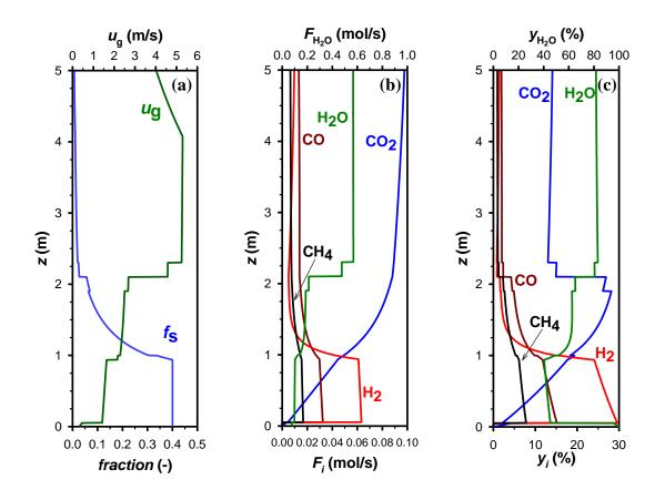
Fig. 4. Axial profiles of (a) solids fraction and gas velocity; (b) flow of gases; and (c) molar fraction of gases ( $N_2$  free). Model prediction for test VII-5.
