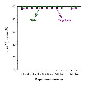
Fig. 8. Efficiency of the carbon separation system,  $\eta_{CS}$ , and efficiency of char recovery in the cyclone,  $\eta_{cyclone}$ , predicted by the model for the different experimental conditions in VII and VIII tests.
