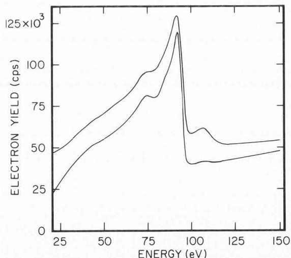
Figure 4: A detailed comparison of the electron-induced and photon-induced Auger yields near the LVV transition of Si. Note the satellite near 106 eV, which is almost completely absent in the electron induced spectrum.
