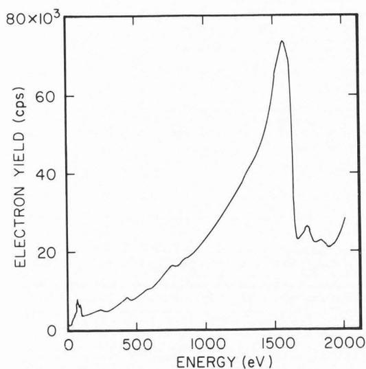
Figure 3: The Auger electron spectrum of 0.3 monolayers of Au on Si (111), using white beam excitation.
