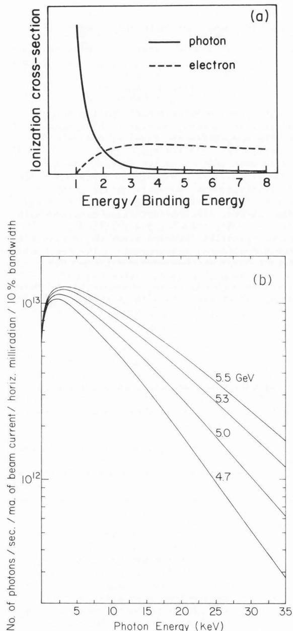
Figure 1: a) Schematic of the ionization cross-sections for electron and photon excitations, from Alford (1979); b) the calculated energy spectrum of the CHES white beam for various stored electron energies.
