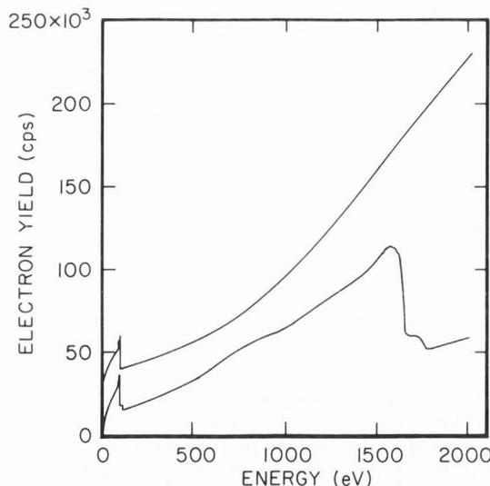
Figure 2: The upper curve is the measured CMA yield for an Auger electron scan from 0 to 2000 eV, using electron excitation at 3 keV and 0.01 microamps; the lower curve was measured using the synchrotron white beam as the excitation source.
