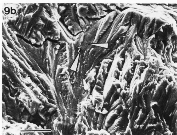
Figs. 9a and 9b: Fatigue striations (arrows) within a fan-like structure, secondary cracks at \Delta K = 400 \text{ N/mm}^{3/2} , f = 0.1 \text{ Hz} .
