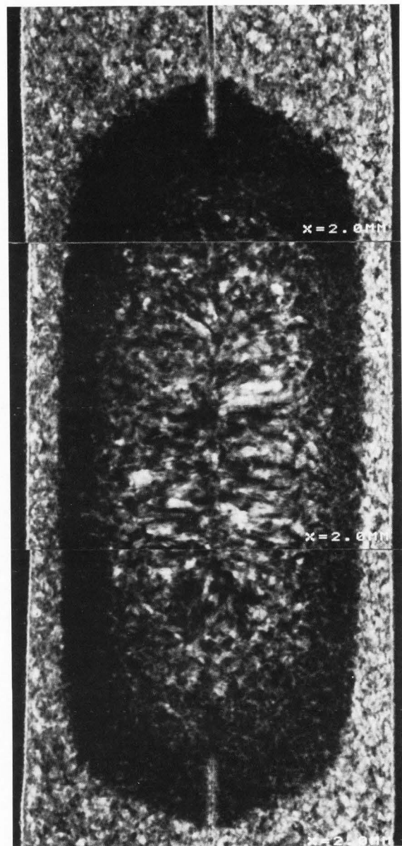
Fig. 2 Cross section of a spot welded junction. The slits mark the interface of the two welded sheets. Acoustomicrograph of the unetched polished surface.
