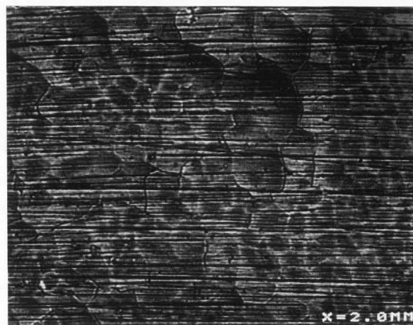
Fig. 12b Subsurface imaging at the same area ( z=-20\mu\text{m} ) shows additional bright contrasted crack-patterns ─── = 100 μm
