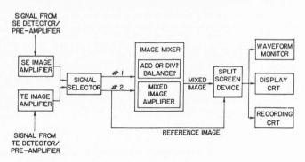
Fig. 1: Block diagram of signal mixing and display system.
