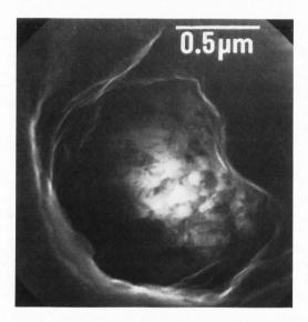
Fig. 5: Higher-magnification mixed TE/SE image taken of dimple in backthinned fracture surface sample.
