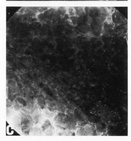
Fig. 6: Micrographs of region of dynamically-compacted Al-6%Si powder sample. a) TE image. b) SE image. Note the ease with which the individual prior particles can be identified. c) Mixed TE/SE image. The mix has been performed to allow the SE component to outline the prior particle boundaries in the TE image.
