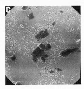
Fig. 11: a) TE, b) SE, and c) mixed TE/SE image of the same region of a sample of powdered coal. The powder particles were held on a holey carbon support film. Notice that particles clinging to the surface of the support film facing away from the SE detector are not visible in the SE component.
