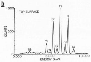
Fig. 10: EDS spectra taken from the particle numbered 2 in Fig. 9c. a) Spectrum with particle on bottom foil surface. b) Spectrum with particle on top foil surface. Note the improvement in the particle-related signal (i.e., the Nb and Ti signals) found in b). (From Allen, 1982.)
