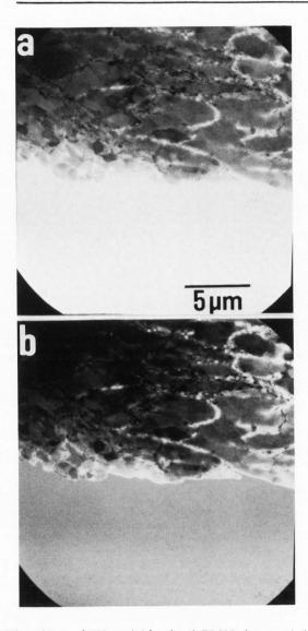
Fig. 12: a) TE and b) mixed TE/SE images taken of the edge of a sample of dynamically-compacted Al-6%Si powder particles. In a) the hole is the brightest object in the image; in b) the signal level of the hole has been reduced by mixing in the SE component. Note the improvement in contrast and image definition in the mixed image near the sample edge.
