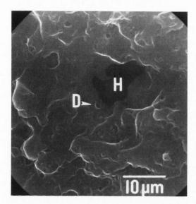
Fig. 3: Low magnification SE image of backthinned fracture surface sample in manganese-modified 316 stainless steel. The hole in the sample produced during thinning has been marked at H. D shows the location of the dimple examined at higher magnifications in Figs. 4 and 5.
