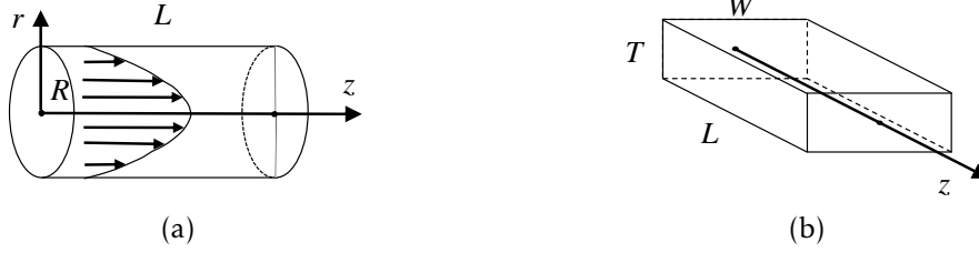
Figure 2.12: Poiseuille velocity profile in a channel with a (a) circular and (b) rectangular cross-section.
