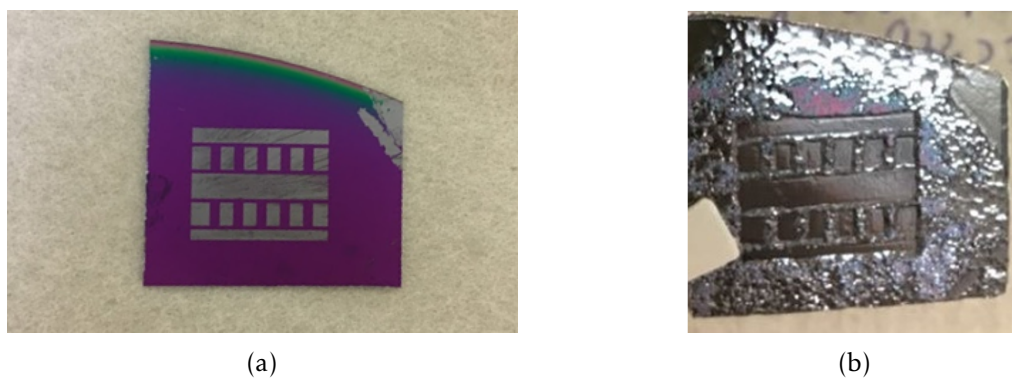
Figure 4.7: (a) Picture of the back side of an unpolished sample after the lithography and RIE and (b) after 1 h of KOH etch.
