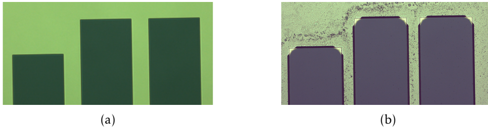
Figure 4.2: Micrographs of (a) printed cantilevers after the first lithography and RIE and (b) the same cantilevers with a thickness of 10 \mu\text{m} after the KOH etch.
