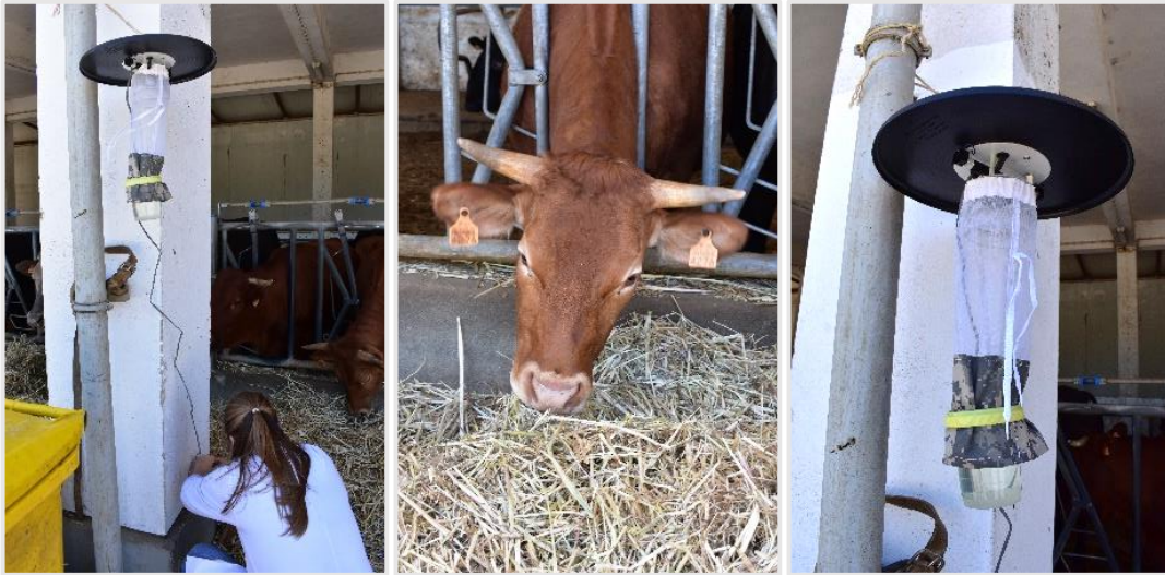
Figure 3.3: Miniature CDC light trap being placed 1,70 m above the ground near domestic cattle in FMV-ULisbon.
