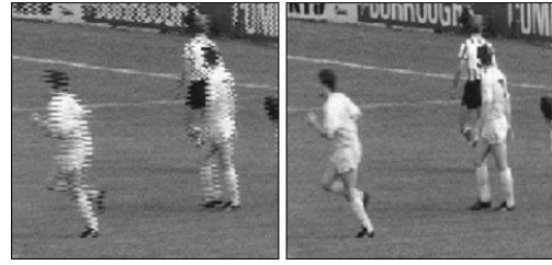
Fig. 8. If picture-repetition is assumed incorrectly, feathering (left) will show.
