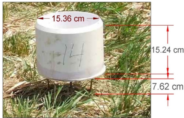
Figure 2. Typical positioning of catch can in the pivot field for uniformity testing.
