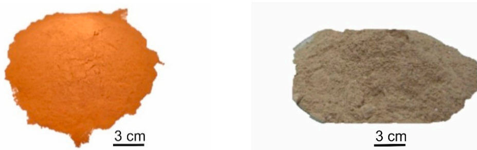
Figure 1. The photograph of sewage sludge incineration ash (FA1; on the left) and FA from incineration of municipal solid waste (on the right).
