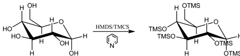
Figure 12 Formation of trimethylsilyl ethers (TMS: –Si(CH 3 ) 3 ). HMDS, hexamethyldisilazane; TMCS, trimethylchlorosilane.
