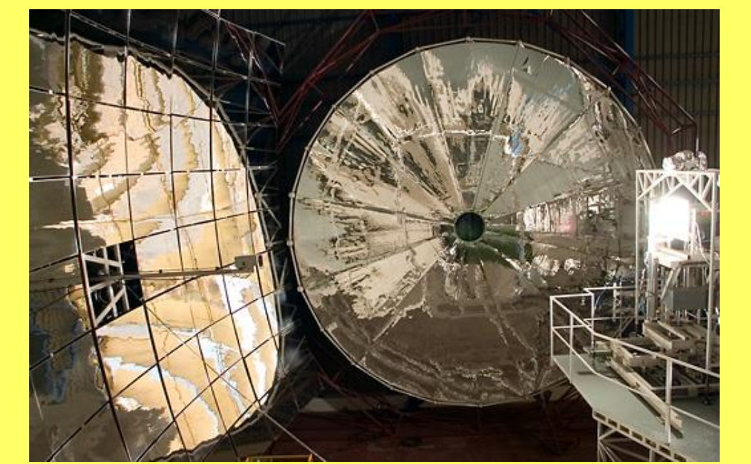
Figure 3. Solar Furnace: Concentrator and receiver in operation at the focus http://www.psa.es/webeng/instalaciones/horno.php
