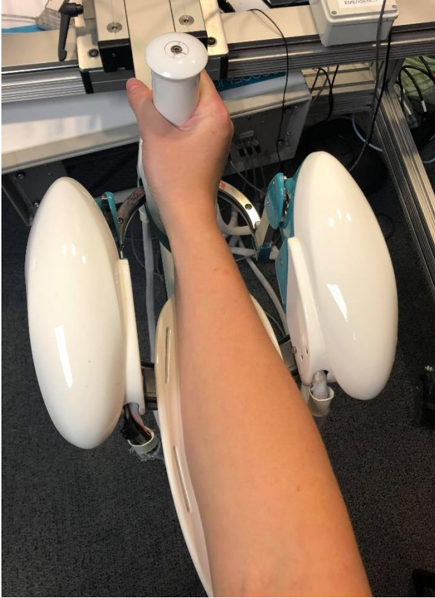
Figure 4. Starting position on Haptic Wrist Device (neutral grip)
