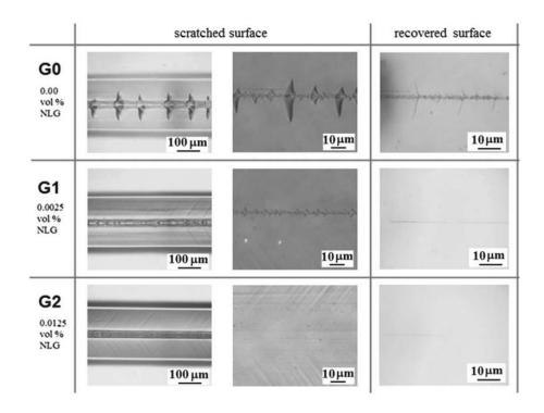
**Figure 20:** Surface images of the as scratched and recovered surfaces. The optical images in the left two columns represent samples after scratch testing. The optical images in the third column are the recovered samples after heating [132].
