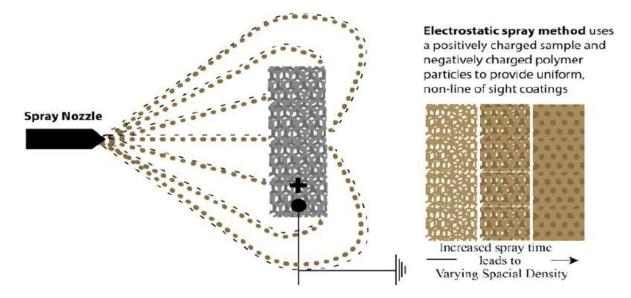
Figure 7: Schematic of electrostatic spray coating process [23].
