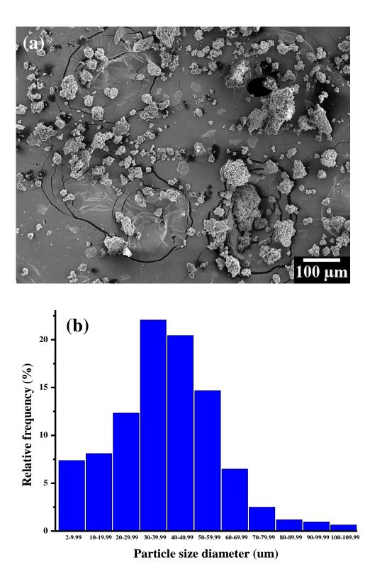
**Figure 59:** (a) SEM micrograph showing varying sizes of SMP epoxy powder processed by ball milling technique, (b) particle size distribution of SMP epoxy powder.
