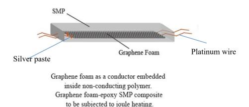
Figure 26: Schematic of a fabricated Electrically Responsive SMP-GrF Composite
