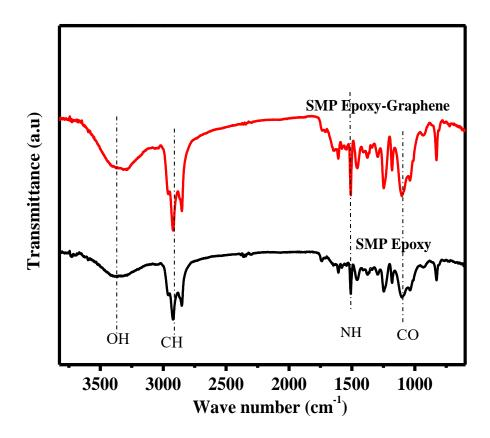
**Figure 66:** FTIR spectra of SMP epoxy and SMP epoxy-0.1 wt.% GNP composite confirming the possibility of interfacial interactions between functionalities on SMP epoxy and graphene
