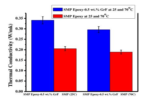
**Figure 38:** Thermal conductivity behavior of SMP Epoxy and SMP epoxy-0.5 wt.% GrF at 25 and 70°C
