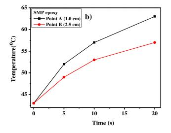
Table 4.0. Thermal gradient of direct heating of SMP epoxy
