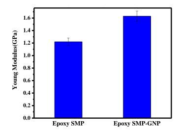
**Figure 71:** (a) Uniaxial tensile stress-strain curves for mold-cast SMP epoxy and SMP epoxy composite of 0.1 wt.% GNP content (b) Comparison of Young modulus of SMP epoxy and composite of 0.1 wt.% GNP content
