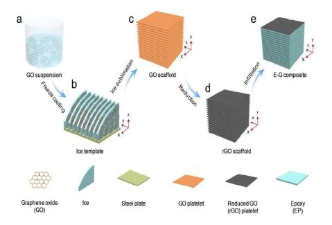
**Figure. 19:** Schematic of the fabrication of E-G composites. (a) Preparation of GO aqueous suspension with THF, then freezing by bidirectional freeze-casting (b). The lamellar GO scaffold was obtained after freeze drying (c). Subsequently, heating was applied to reduce the GO scaffold, forming an rGO scaffold (d). Finally, the E-G composite was produced by infiltrating with shape memory EP and (e) curing [125].
