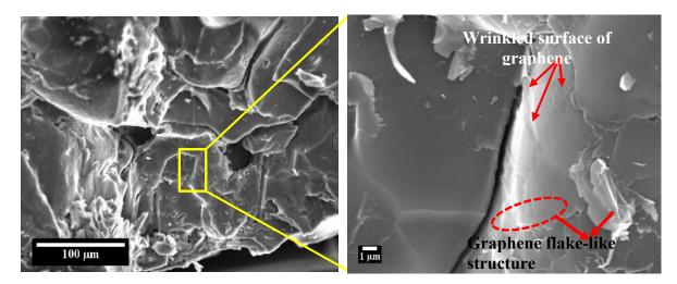
**Figure 28:** Fracture surface of SMP epoxy-GrF composites revealing wrinkled graphene surface and graphene flake-like structure at (a) low and (b) high magnifications
