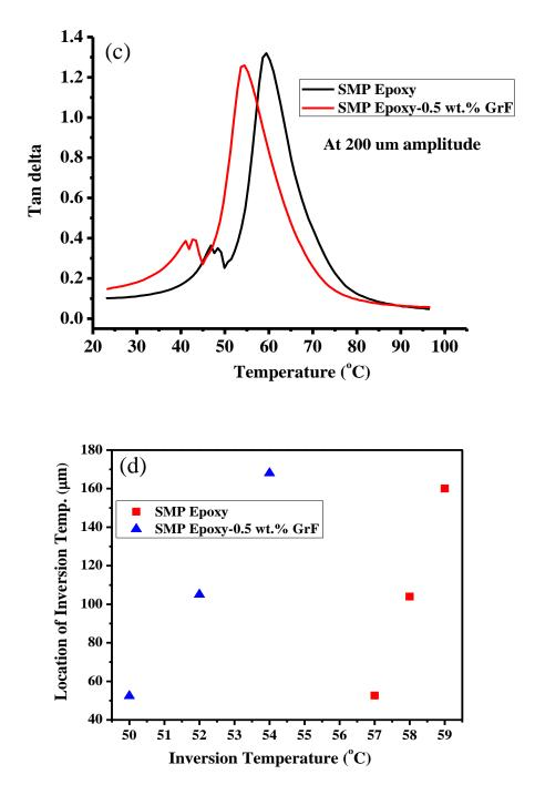
**Figure 54:** Plot of loss tangent versus temperature of SMP epoxy and SMP epoxy-0.5 wt.%GrF at amplitude of (a) 50  $\mu$ m (b) 100  $\mu$ m and (c) 200  $\mu$ m; (d) Plot of distance points against inversion temperature of SMP Epoxy and SMP Epoxy-0.5 wt.% GrF
