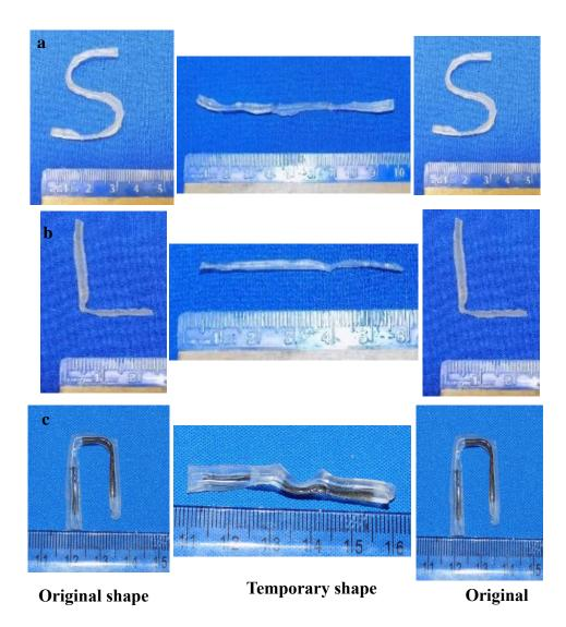
**Figure 43:** a) Images of epoxy SMP fabricated to S-shape, deformed to thin rectangular shape and recovered back to S-shape under the influence external heat stimulus; b) Images of epoxy SMP designed to L-shape. deformed into rectangular shape and recovered back to L-shape when subjected to heat trigger; c) Images of graphene foam-epoxy SMP made into inverted U-shape deformed into irregular rectangular shape and recovered back to inverted U-shape when stimulated by heat
