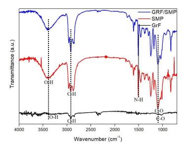
**Figure 30:** FTIR spectra of GrF, SMP epoxy and SMP epoxy-GrF composite confirming possibility in interfacial interactions between functional groups on SMP epoxy and GrF
