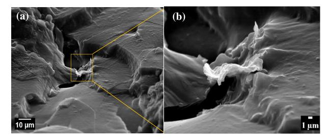
**Figure 74:** SEM images of the fracture surface showing the crack-bridging mechanism in SMP epoxy-GNP composite. (a) low magnification of  $1500 \times$  and (b) high magnification of  $5000 \times$
