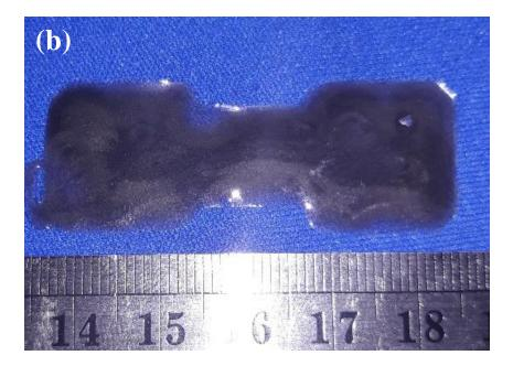
**Figure 62:** Images of 3D printed dog-bone shape sample placed under nearly cryogenic condition. a) SMP epoxy b) SMP epoxy-0.1 wt.% GNP
