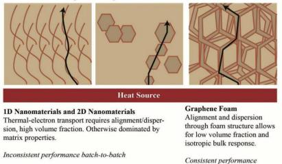
Figure 13: Scheme of thermal and electron transport in composites reinforced with 1D, 2D and 3D GrF [23].
