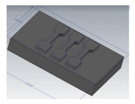
Figure 24: Reverse impression dog-bone mold fixture
