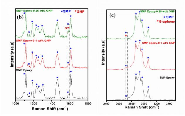
**Figure 65:** Raman spectrum of (a) GNP powder [158]; Raman spectra of SMP epoxy, SMP epoxy-0.1 wt.% GNP and SMP epoxy-0.25 wt.% GNP at (b) wavenumber 1000 - 1800 cm<sup>-1</sup>; (c) at wavenumber 2000 - 4000 cm<sup>-1</sup>.
