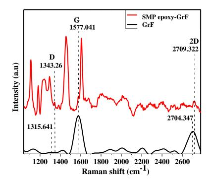
**Figure 29:** Raman spectrum of GrF and SMP epoxy-GrF Composite revealing peaks characteristics of GrF and peak shifts in the composite
