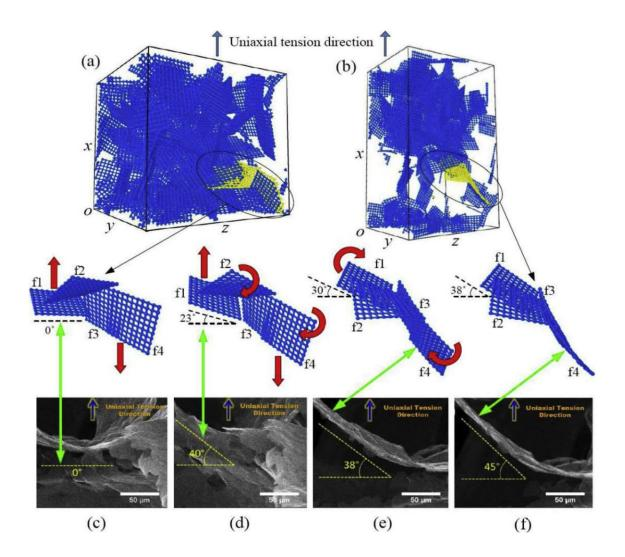
**Figure 5:** Meso-structure evolution during tensile deformation. (a) Beginning state of GrF in uniaxial tension (b) End state of GrF uniaxial tensile deformation; Yellow color represents local graphene flakes. (c-f) four sequential thermodynamic states of mesostructures during tensile deformation [73].
