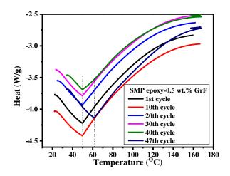
**Figure 40:** Glass transition behavior of SMP epoxy-0.5 wt.% GrF as a function of T-M cycles
