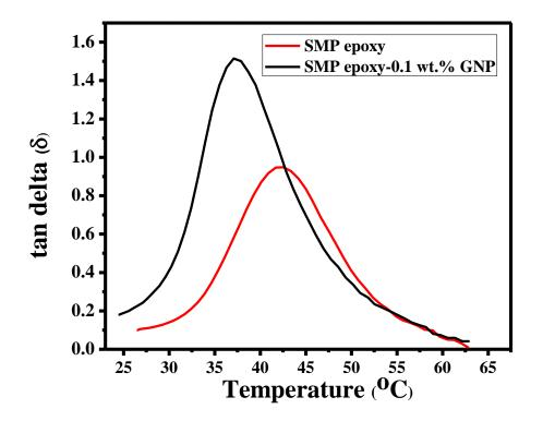
**Figure 75:** Plot of (a) storage modulus and (b) tan delta of SMP epoxy and SMP epoxy-0.1 wt.% GNP composite at amplitude load of 5  $\mu m$
