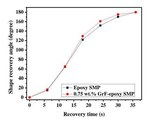
**Figure 36:** Shape recovery angle as a function of time for SMP epoxy and -SMP epoxy-0.75 wt.% GrF composite injected with hot air from the heat gun
