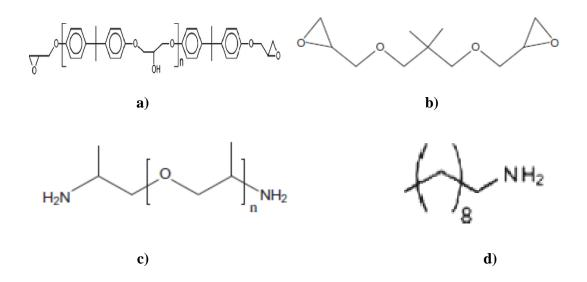
**Figure 16:** Chemical Structures of SMP epoxy components (a) Diglycidyl ether bisphenol A (DGEBA); (b) Neopentyl glycol diglycidyl ether (NGDE); (c) Jeffamine D-230 (n~2.5); (d) decylamine [118].
