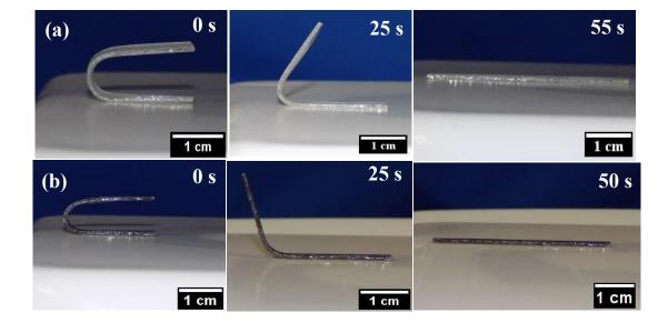
**Figure 33:** Shape recovery images of (a) SMP epoxy and (b) SMP epoxy-0.75 wt.% GrF composite triggered by direct heating from the hot plate.
