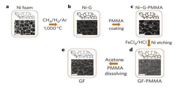
**Figure 3:** Synthesis of Graphene foam: (a and b) CVD growth of graphene films (Ni-G, b) using a nickel foam as scaffold. (c) as-grown graphene film after coating a thin PMMA supporting layer (Ni-G-PMMA). (d) Graphene foam coated with PMMA (GrF-PMMA) after etching the nickel foam with FeCl<sub>3</sub>/HCl solution. (e) Free-standing GrF after PMMA dissolution with acetone [67].
