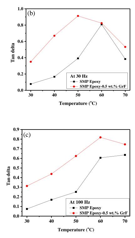
**Figure 52:** Plot of loss tangent versus of SMP Epoxy and SMP Epoxy-0.5 wt.% GrF a) as a function of number of cycles; as a function temperature at b) 30 Hz; c) 100 Hz
