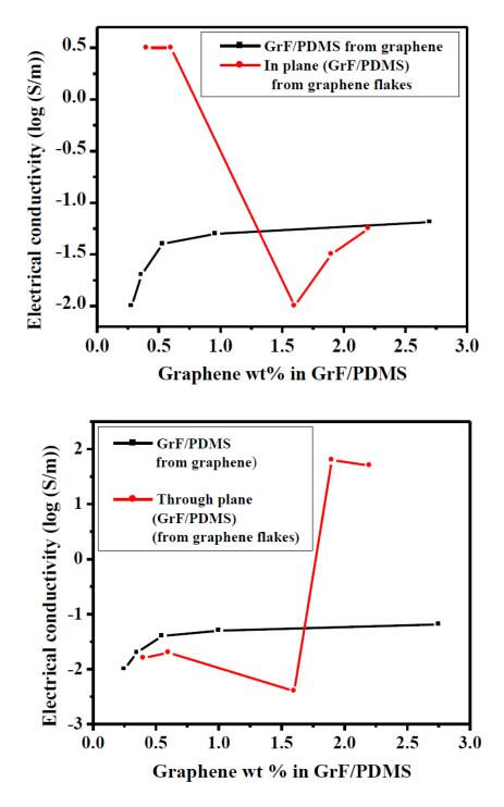
**Figure 11:** (a). Electrical conductivities of GrF/PDMS (in-plane) vs Graphene wt.%. (b) Electrical conductivities of GrF/PDMS (through-plane) vs Graphene wt.% [23].
