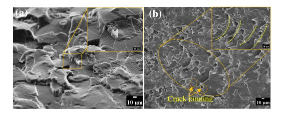
**Figure 73:** SEM fractographs of SMP epoxy-GNP composite. (a) image taken from perpendicular planes to the layer deposition axis, with  $2200 \times [inset]$  (b) image taken from parallel plane to the layer deposition axis, with  $750 \times [inset]$
