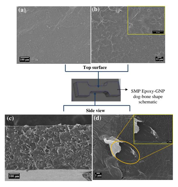
**Figure 64:** SEM micrographs of cross-section of 3D printed dog-bone shape specimen from SMP epoxy-0.1 wt.% GNP (a) at lower magnification ( $150\times$ ); (b) at higher magnification ( $1500\times$  and  $5000\times$  [*inset*]) and SMP epoxy-0.1 wt.% GNP (c) revealing rough surfaces and (d) interface between graphene and SMP epoxy
