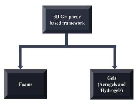
Figure 2: Classification of 3D Graphene-based frameworks [23].
