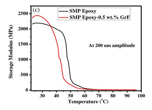
**Figure 53:** Plot of storage modulus versus temperature of SMP epoxy and SMP epoxy-0.5 wt.% GrF at an amplitude of (a) 50  $\mu m$  (b) 100  $\mu m$  and (c) 200  $\mu m$
