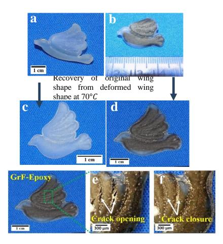
**Figure 46**: (a) Images of deformed (temporary shape) wings of SMP epoxy-GrF bird and (b) SMP epoxy-GrF bird at  $25^{\circ}C$ ; (c) Images of recovery of the deformed wings of SMP epoxy bird and (d) SMP epoxy-GrF SMP bird (e) Image of cracked-open wing of biomimetic SMP epoxy-GrF bird after  $15^{\text{th}}$  T-M cyclic deformation.; (f) Images of the crack-closed wing of SMP epoxy-GrF bird
