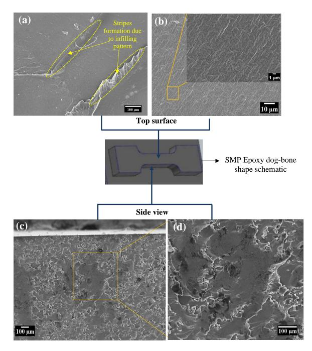
**Figure 63:** SEM micrographs of cross-section of 3D printed dog-bone shape specimen from SMP epoxy top view surface (a) at lower magnification  $(150\times)$ ; (b) at higher magnification  $(1500\times \text{ and } 5000\times [inset])$  and side view surface (c) at lower magnification  $(100\times)$  and (d) at higher magnification  $(750\times)$
