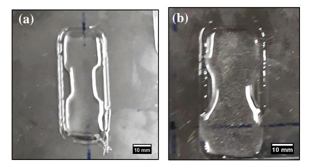
**Figure 61:** Image of 3D printed dog-bone shape sample using partial cured SMP epoxy precursor. (a) immediately after printing (retaining the dog-bone shape geometry); (b) 30 minutes after printing (revealing smudging of SMP epoxy and not maintaining the shape geometry)
