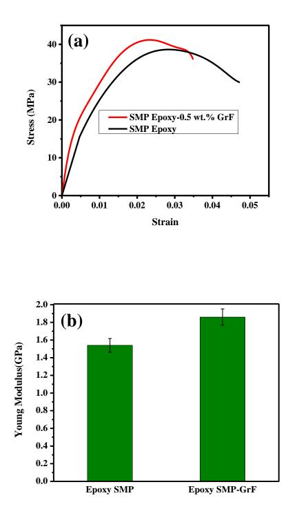
**Figure 47:** (a) Uniaxial tensile stress-strain curves for SMP epoxy and mold cast composite of 0.5 wt.% GrF content (b) Comparison of Young modulus (elastic modulus) of SMP epoxy and composite of 0.5 wt.% GrF content.
