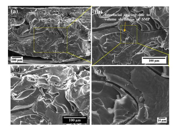
**Figure 48:** SEM images of the fracture surface of SMP epoxy-GrF composite. (a) GrF branch-node anatomy retaining its integrity in SMP epoxy after curing (b) shrinkage of SMP epoxy leading to the interfacial spacing between GrF and SMP epoxy (c) distinct surface features of GrF and SMP epoxy showing higher magnification of the interfacial spacing (d) close view of good interface regions between GrF and SMP epoxy.
