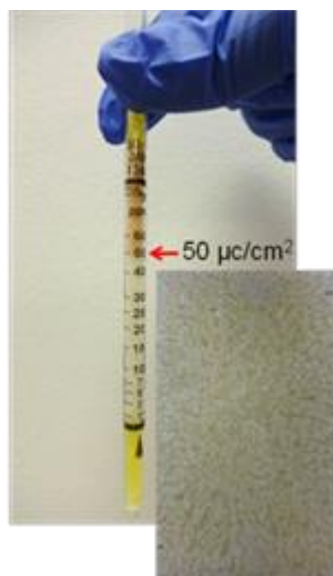
Figure 3.9. Measurement of the Chloride Contamination Level.
