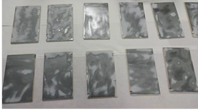
Figure 3.8. Hand Cleaned Steel Panels (Three-coat System).
