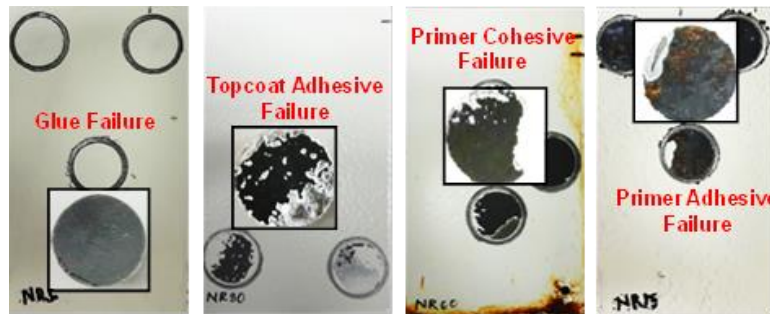
Figure 5.8. Different Failure Modality of Pull-Off Strength for NPE-ZRP Coupons.
