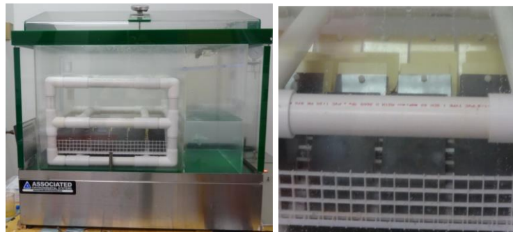
Figure 3.3. Test setup for Salt-fog Exposure.
