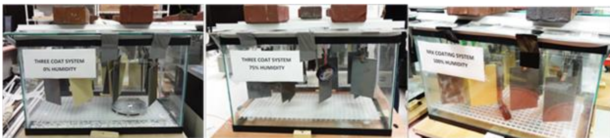
Figure 3.10. Humidity Chamber for Test Panel Exposure.
