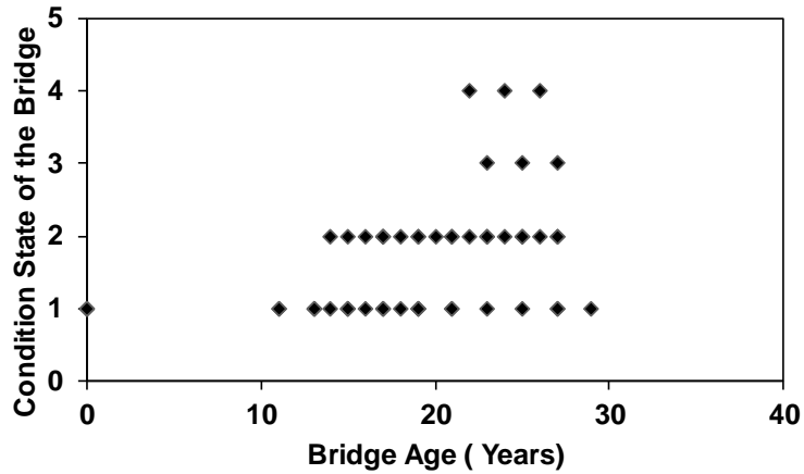
Figure 2.8. Bridge Condition State over Age (FDOT Bridge Inspection Report).
