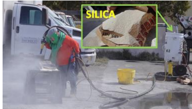
Figure 3.6. Sandblasting of the Coupons (Plain Steel Coupon).
