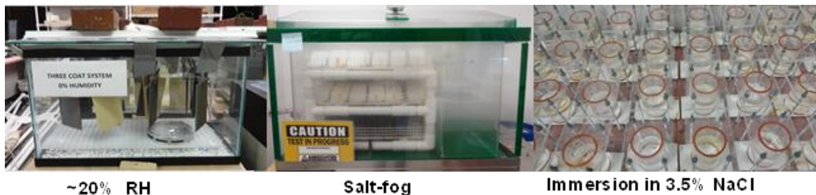
Figure 3.14. Cyclic Wet/Dry Exposure in Three Different Condition (20 Cycles).
