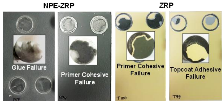
Figure 4.3. Different Coating Failure Modality.
