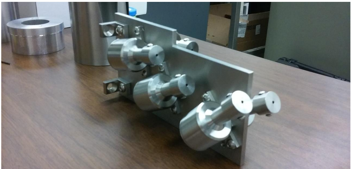
Figure 29. Machined 6-detector probe head (stainless steel SS316).
