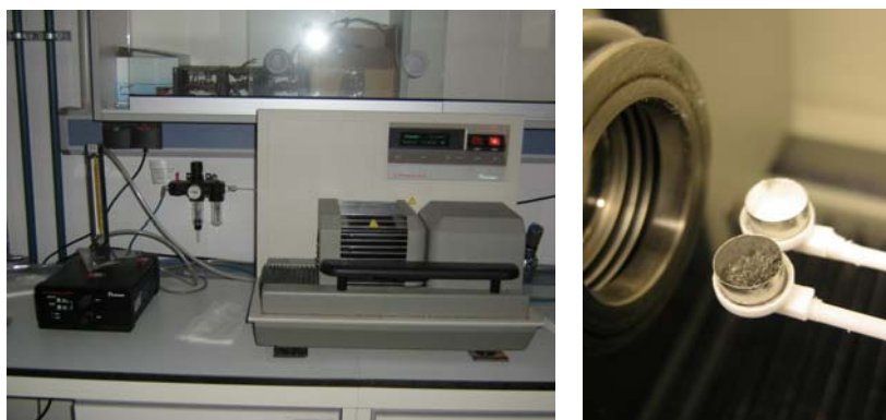
Figure 2.9. Simultaneous Differential Thermal Analysis Module SDT 2960 and gas flow controller (left). Platinum cups on the balance arms.
